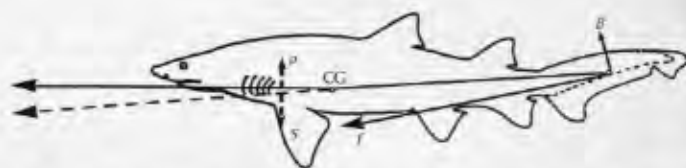
Figure 11.3. Profile of a shark showing the forces generated by the tail in swimming. The line of net thrust from the tail is directed through the center of gravity (CG). This produces a net sinking effect S that is offset by a lifting effect P from the planing action of the pectoral fins. B and F , resolution of force from the tail into lift and a forward force, respectively. From Thomson (1976).
