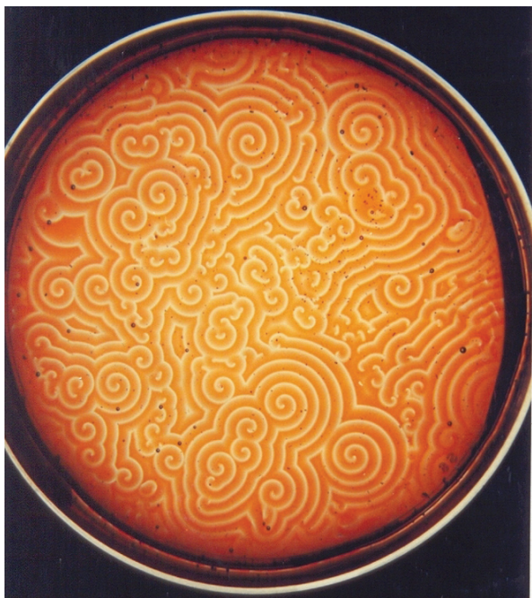
Fig. 2.3 Formation and growth of helical structures (spiral-waves) formed during the Belousov-Zhabotinskii reaction. In the vicinity of a right-handed helix, a left-handed helix is formed, moving synchronously. The photo was taken 40 min after mixing aqueous solutions of 0.33 \text{ mol L}^{-1} malonic acid, 0.33 \text{ mol L}^{-1} \text{NaBrO}_3 , 0.2 \text{ mol L}^{-1} \text{H}_2\text{SO}_4 , and putting them onto a petri dish covered with a 1.4 mm gel produced by 5 mL filtered 14% (w/w) \text{Na}_2\text{O} \times \text{SiO}_2 and 2 mL 25 \text{ mmol L}^{-1} ferroin solution. Gel formation was induced by adding 1.2 mL of 1.4 \text{ mol L}^{-1} \text{H}_2\text{SO}_4 . The diameter of the petri dish is 85 mm. Photo: Christoph Gottschling, Dept. Phys. Chemistry, University of Bremen
